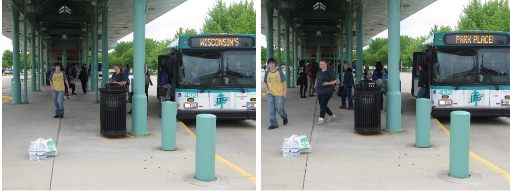
Overhead rotating destination signs, which show longer messages by alternating between two readings on a vehicle, are used on school trippers.
