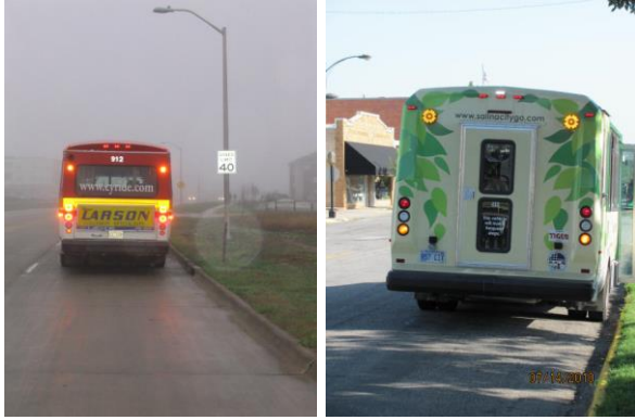
Left: Reflective stripe and flashers. Right: Flashers located high on the vehicle.
