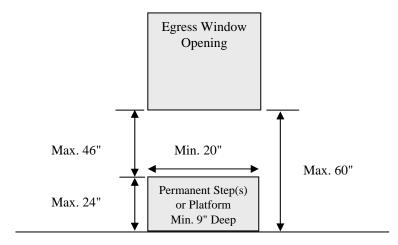
If a window is provided as an exit located below grade, then an areaway shall be provided. The width of the areaway shall be at least equal to the width of the exit window, the bottom of the areaway shall not be more than 46" below grade, shall be a minimum of three feet measured perpendicular from the wall, and shall be constructed to prevent rainfall flowing into the areaway from entering the dwelling.
