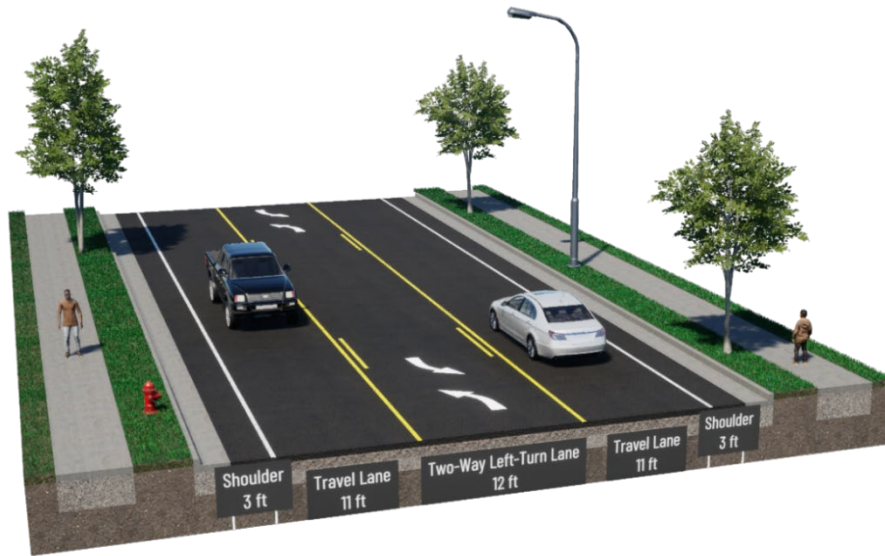
Figure 2-3, Alternative 2: 3-Lane Corridor, with Narrow Shoulders
