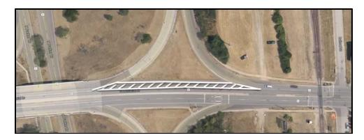
2. In the gore area of the merge, it is suggested adding edgeline pavement marking along the lane edges of the ramp and Memorial Dr., chevron pavement marking in the neutral area, and a dotted edgeline extension. These markings are expected to reinforce the message that a merge is coming up.
