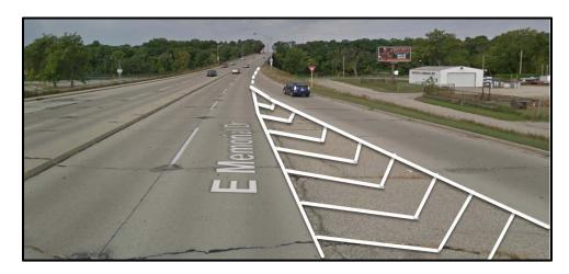
3. To further reinforce the message that a merge is impending, it is suggested adding a supplemental text warning sign stating "MERGE AHEAD" to the existing merge sign and adding a second set of signs on the outside shoulder of the ramp.
