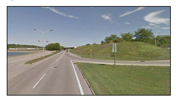
It is suggested that the lane-drop improvement #1 listed for the SB to WB ramp also be considered at this location. At this location, if it is feasible to drop the outside lane as an exit only to the NB to EB ramp, then the EB to NB ramp could become a free-flow on-ramp and reestablish the outside lane on northbound Parker Dr.
